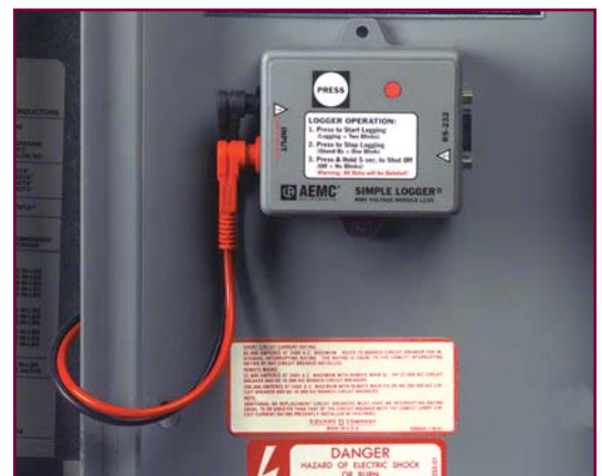
Model L230 monitoring the line voltage on an injection molding machine
