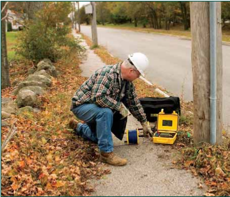
Model 6470 quickly checks ground rod resistance with its Connect – Press – Read approach
