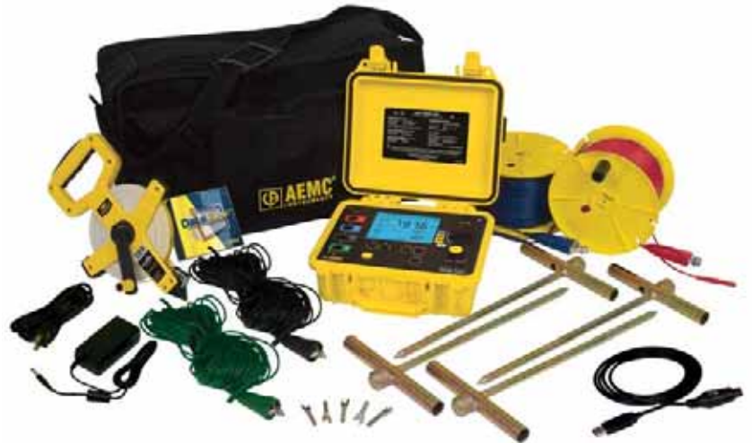
Multi-Function Ground Resistance Tester Model 6470 Kit (500 ft kit shown) Includes meter, NIMH batteries, optically isolated USB cable, DataView® software, external battery charger, AC power cord, one 30 ft green wire, one each 500 ft red and blue wire, one each 100 ft black and green wire, set of five spade lugs, four 14.5" auxiliary electrodes, tape measure, carrying case and user manual Catalog #2135.04
